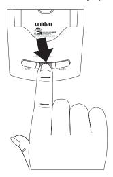
When Audio Alert Only is selected, the visual alert and signal strength meter are disabled. In this mode, all lighted LEDs will dim. Press the AUDIO button again for the Full Alert (audio and visual) Mode. (Do not set the Volume control at minimum when in Audio Alert Only because there will be no alert.)
